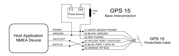
Figure 3. Basic NMEA Device Interconnection
